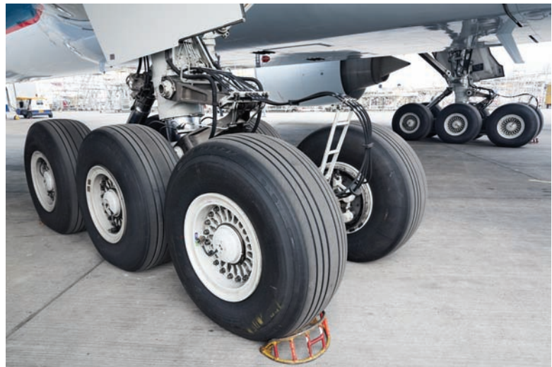
FIGURE 1-10 Landing gear for a large aircraft (Shutterstock)
