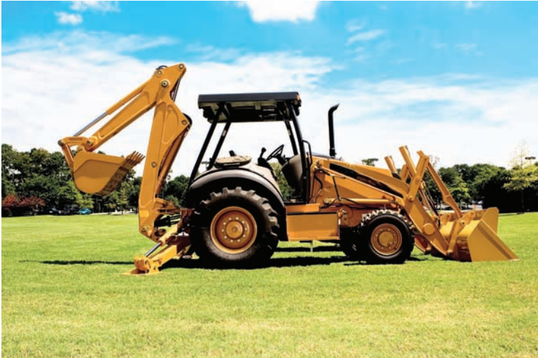
FIGURE 1-6 Construction backhoe and front-end loader (Shutterstock)
